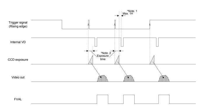
Note 1: The video output will be V reset by the next internal HD signal immediately after the exposure is finished. Note 2: The exposure time is set by the preset electronic shutter speed.
